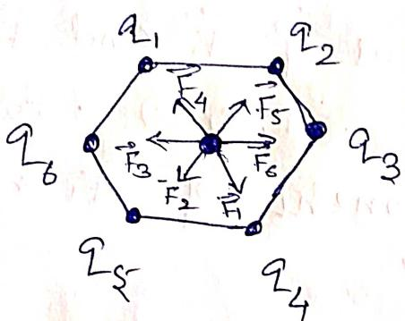
Like charges repel, so the force on the central particle due to any one of the other charges will point directly away from that charge. Since all charges are equal and the distance from the center to each vertex is the same, each of the force contributions from the outer six charges will have the same magnitude.
